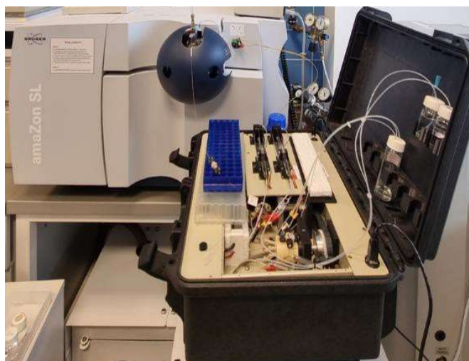
Figure 1. Miniaturized chromatographic system connected to ESI-MS instrument.
